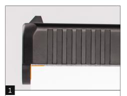
Complete the Safety check and Field Strip steps as indicated in the GLOCK Instructions for use. Place the slide of your pistol on a flat surface making sure that the recoil spring guide ring overlaps the surface.
