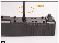
Tighten the 2 screws to fix the GLOCK MOS Adapter Plate on your GLOCK MOS Pistol. Screws should be tightened to a secure hold. (Attention: The set includes 2 additional replacement screws. It is not recommended to use these screws to fix the optical system itself.)
